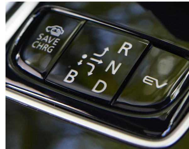
» (ABOVE) REGENERATIVE BRAKING Regenerative braking uses kinetic energy to charge the drive battery when the accelerator is released and while the brake pedal is being pressed.
