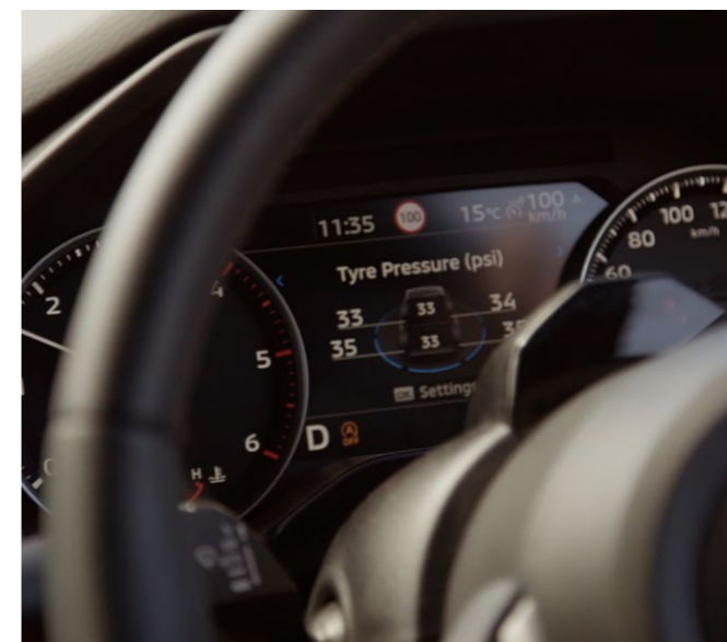
» TYRE PRESSURE MONITORING SYSTEM Check tyre pressures without leaving the cabin.
